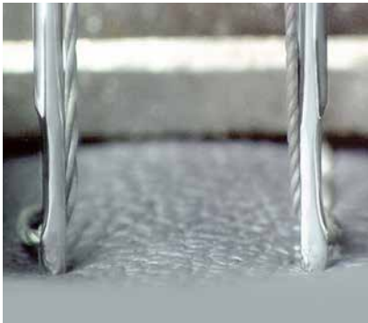
Different threading direction for right and left needle
